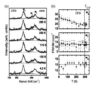
FIG. 5. Raman spectra of CFO for a few selected temperatures (shown by the side of the spectrum) in the spectral window  $650-1000 \text{ cm}^{-1}$ . The dotted lines show Lorentzian fits to the data, which were resolved into three peaks, i.e.,  $W_6$ ,  $W_7$ , and  $W_8$ . (b) The variation of the FWHMs with lowering of temperature.
