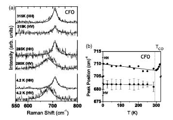
FIG. 4. (a) The HH and HV polarized spectra of the  $W_5$  mode of CFO at a few temperatures. The solid lines are Lorentzian fits to the data. (b) The variation of  $W_5$  mode as a function of temperature. The mode splits into a high-frequency (HH-polarized) and a low-frequency mode (HV-polarized) below  $T_{co}$  (290 K).
