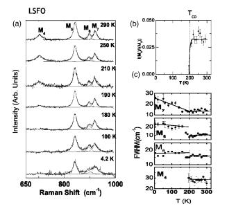
FIG. 7. Raman spectra of LSFO for a few selected temperatures (shown by the side of the spectrum) in the spectral window  $650-1000 \text{ cm}^{-1}$ . The dotted lines show Lorentzian fits to the data, which were resolved into four peaks, i.e.,  $M_4$ ,  $M_5$ ,  $M_6$ , and  $M_7$ . (b) Intensity of the  $M_4$  peak normalized to that of the  $M_5$  with lowering of temperature and (c) variation of FWHMs with lowering of temperature.
