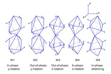
FIG. 2. Vibrational pattern of the Raman active modes assigned to  $W_1$ ,  $W_2$ ,  $W_3$ ,  $W_4$ , and  $W_5$  for CFO.
