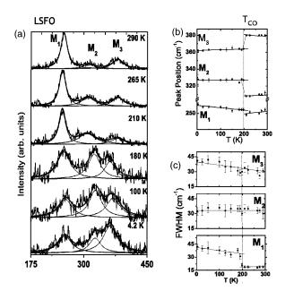
FIG. 6. Raman spectra of LSFO for a few selected temperatures (shown by the side of the spectrum) in the spectral window  $175-450 \text{ cm}^{-1}$ . The dotted lines show Lorentzian fits to the data, which were resolved into three peaks, i.e.,  $\mathbf{M}_1$ ,  $\mathbf{M}_2$ , and  $\mathbf{M}_3$ . (b) Variation of peak positions and (c) FWHM with lowering of temperature.
