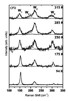
FIG. 3. Raman spectra of CFO for a few selected temperatures (shown by the side of the spectrum) in the spectral window  $100-350 \text{ cm}^{-1}$ . The dotted lines show Lorentzian fits to the data, which are resolved into four peaks, i.e.,  $\mathbf{W}_1$ ,  $\mathbf{W}_2$ ,  $\mathbf{W}_3$ , and  $\mathbf{W}_4$ .
