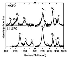
FIG. 1. Room temperature, i.e., 300 K Raman spectra of (a) CFO and (b) LSFO. The dotted lines are Lorentzian fits to the data. The CFO spectrum can be resolved into eight modes while the LSFO spectrum can be resolved into seven modes. The corresponding modes are labeled in the figure.
