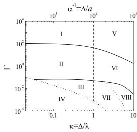
Regions III (VII and VIII) correspond to Coulomb (Yukawa) ideal gases. The range of dust-dust interaction is smaller than the intergrain distance and only pair collisions are important. In addition, in the region VIII the pair Yukawa interaction asymptotically reduces to the hard sphere limit, forming a "Yukawa granular medium". In region IV the electrostatic interaction is unimportant and the system is like a usual granular medium.
