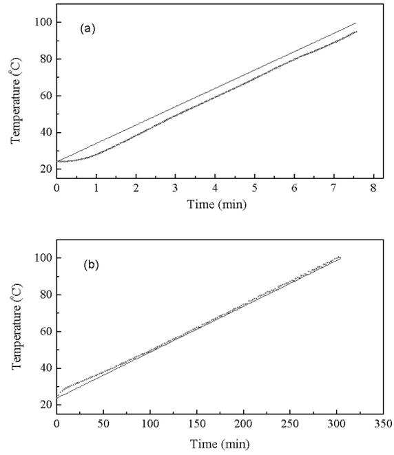
**Fig 3.** Performance of the controller during (a) 10°C/min and (b) 0.25°C/min heating ramps
