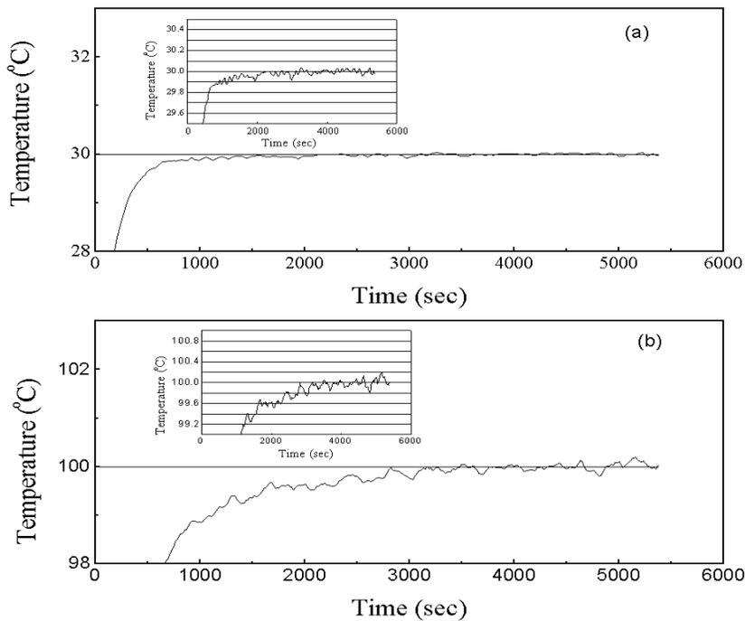
**Fig2.** Performance of the controller for (a) 30°C and (b) 100°C. The instantaneous temperature  $T_c$  and the Set Temperature  $T_s$  are recorded over a period of 90 minutes
