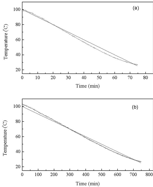
**Fig 4** Performance of the controller during (a) 1°C/min and (b) 0.1°C/min cooling ramps
