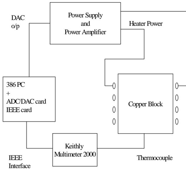
**Fig 1.** Block Diagram of the Temperature Control System
