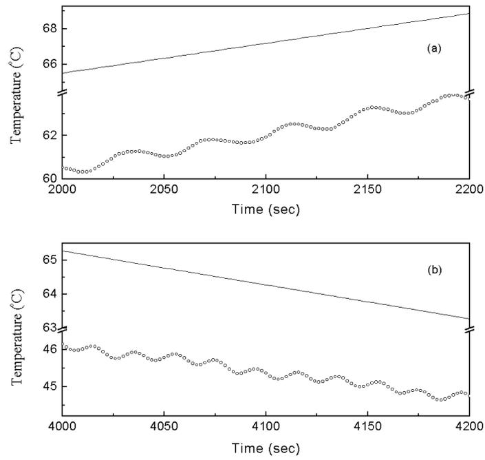
**Fig 5.** Modulation in Temperature superimposed on (a) Heating and (b) Cooling ramps. A lead / lag between the programmed ramp indicated by straight lines and the modulated variation in temperature indicate by open circles can also be seen
